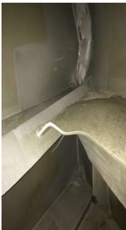
Renew brackets connection for SL 22.4 to SL 22.6, 12mmt 900 x 600 x 3pcs
