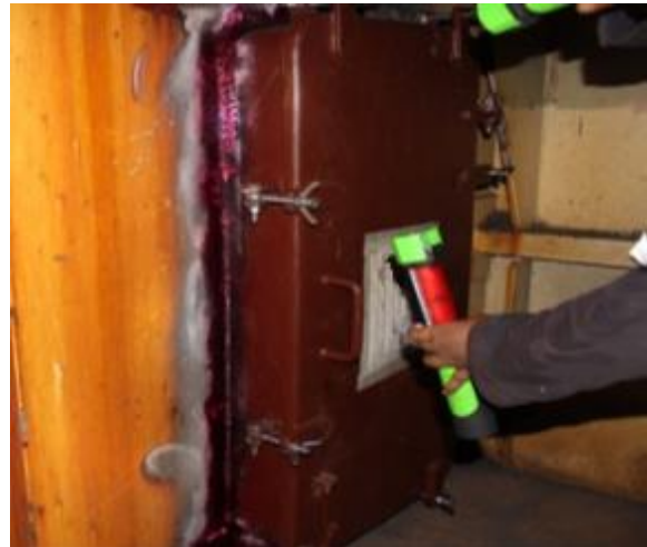
DPI Test carried out on all 3 locations and witnessed satisfactory by C/O
