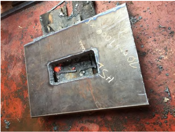
New Material pre-cut in workshop. Marked and pre-fabricate on-site based on existing masurement.
