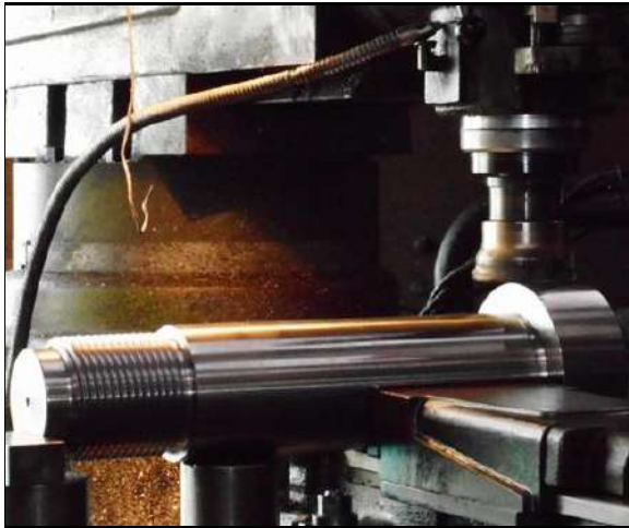
Milling Spanner Faces on Bolt Head (23.11.17)
