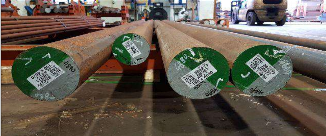
Round Bar, Unmachined AISI 4140 (Heat No : 384277) (21.11.17)
