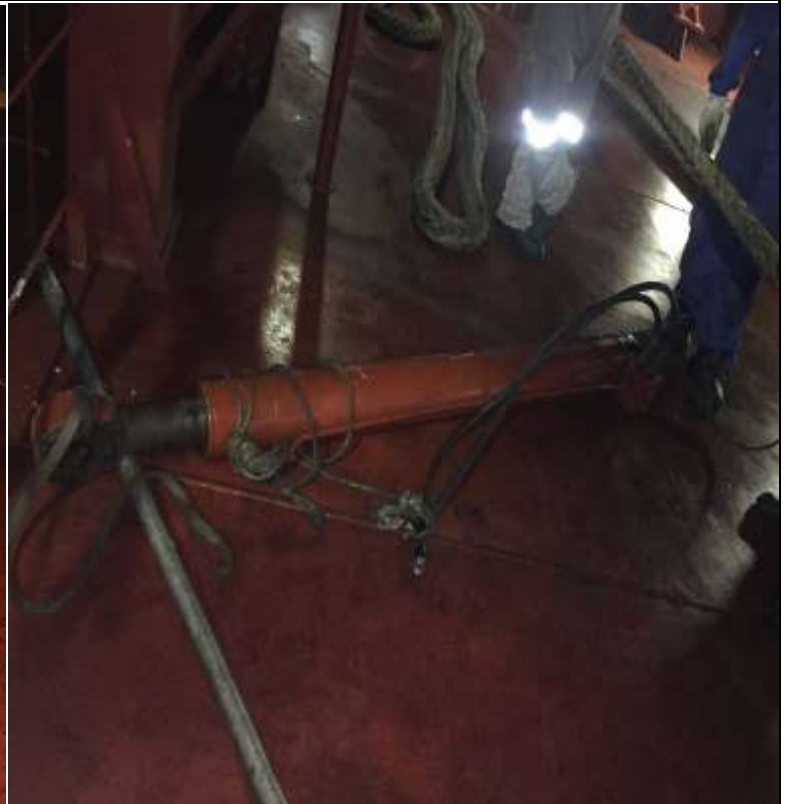
Lifting Hydraulic Cylinder manually in place after thorough cleaning of hinges
