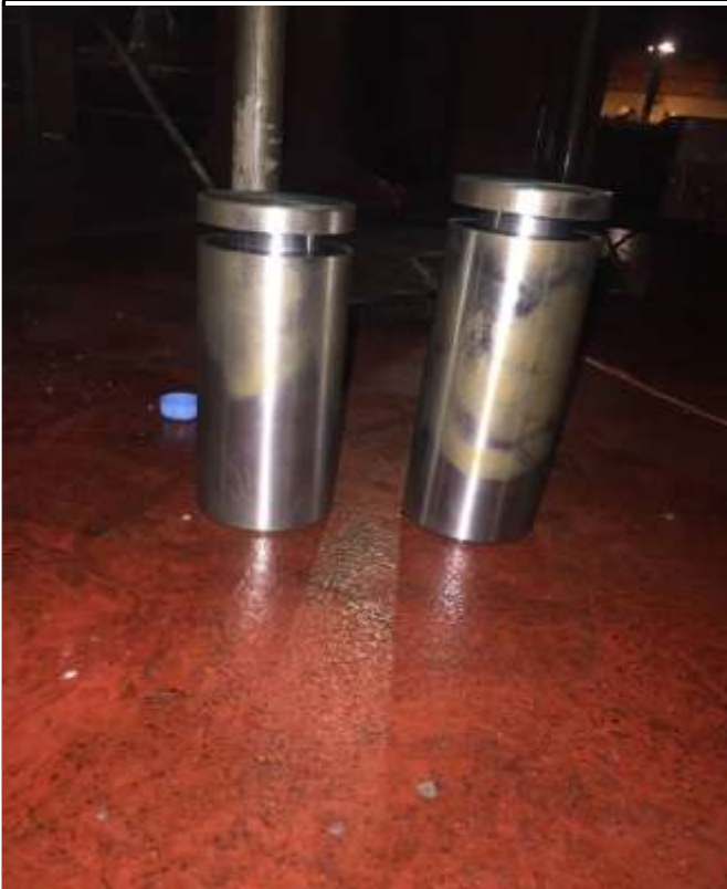
Lifting Hydraulic Cylinder manually in place after thorough cleaning of hinges
