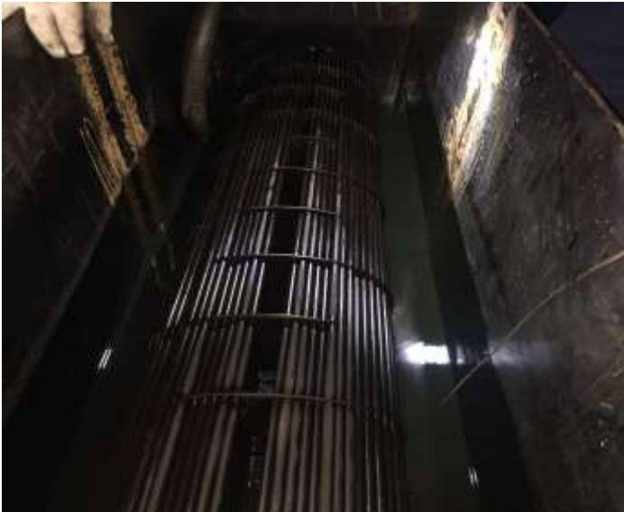
Heating bundle going through the first stage chemical ultrasonic cleaning
