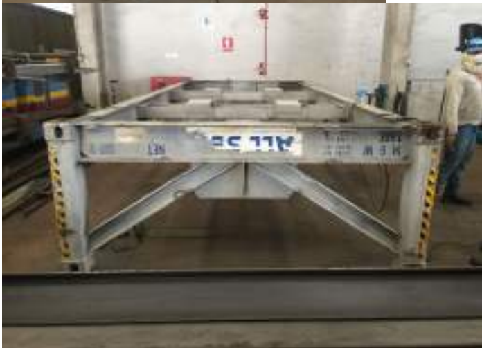
Re-adjusted & aligned corner casting vertical legs to main frame of flat rack
