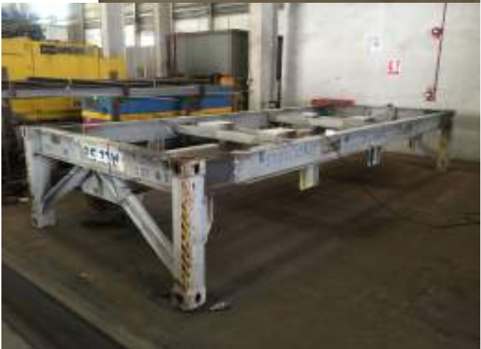
Re-adjusted & aligned corner casting vertical legs to main frame of flat rack
