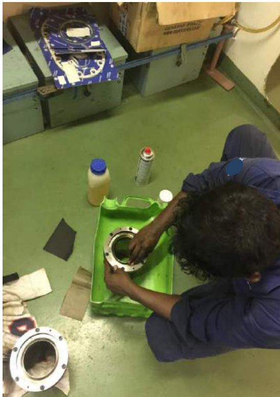
↙ ↘ Overhauling of piston and linear units
