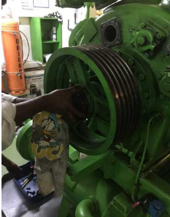
To remove the pulley, sleeve and seal for overhaul works
