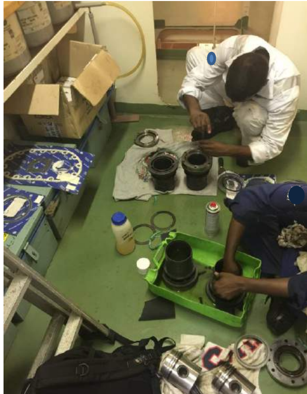
↙ ↘ Overhauling of piston and linear units
