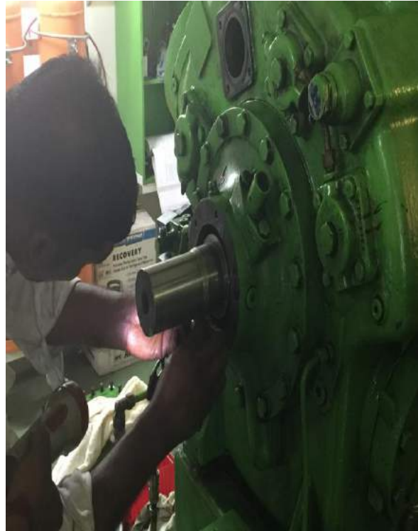
To remove the pulley, sleeve and seal for overhaul works
