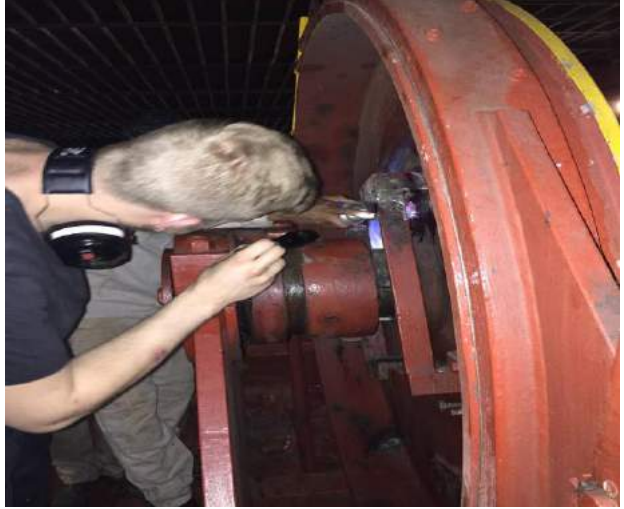
2nd Engineer carried out winch operational test, no defects found.
