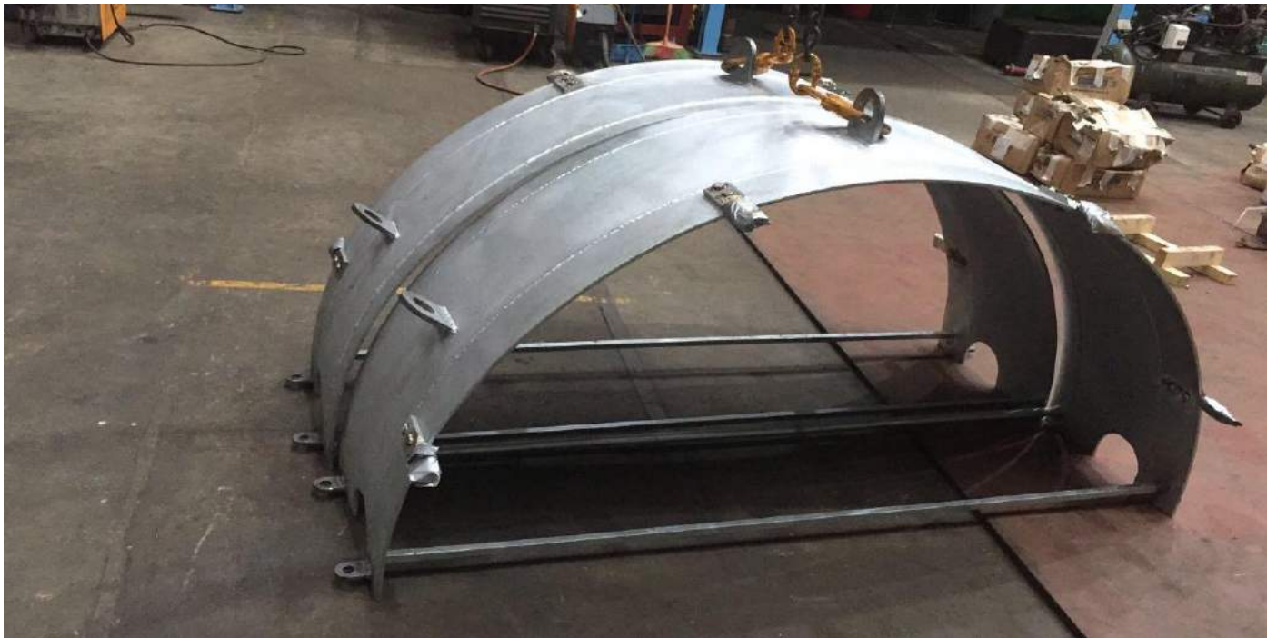
↑ Pre-fabricated Rope Guard in HSD Workshop
