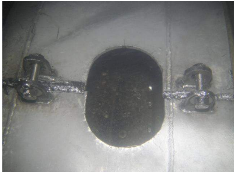
Upon completion of full welding securing Rope Guard, Operation photos and videos were submitted to Chief Officer/Master and acknowledged work to be satisfactory.
