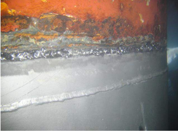
Position of new Rope Guard well secured and carried out full welding
