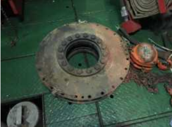
Assembled vulkan coupling connecting to shaft of generator
