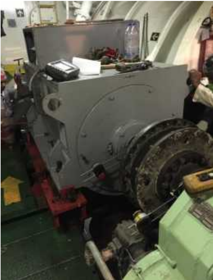
Laser alignment in progress
