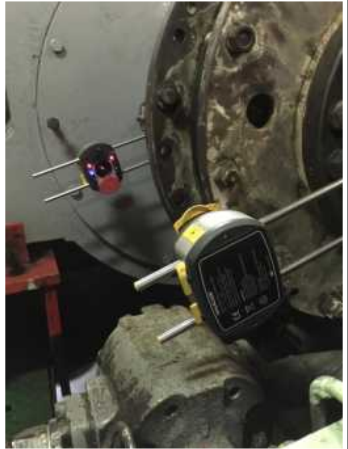
Laser alignment in progress
