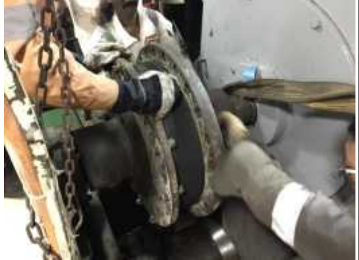
Assembled vulkan coupling connecting to shaft of generator
