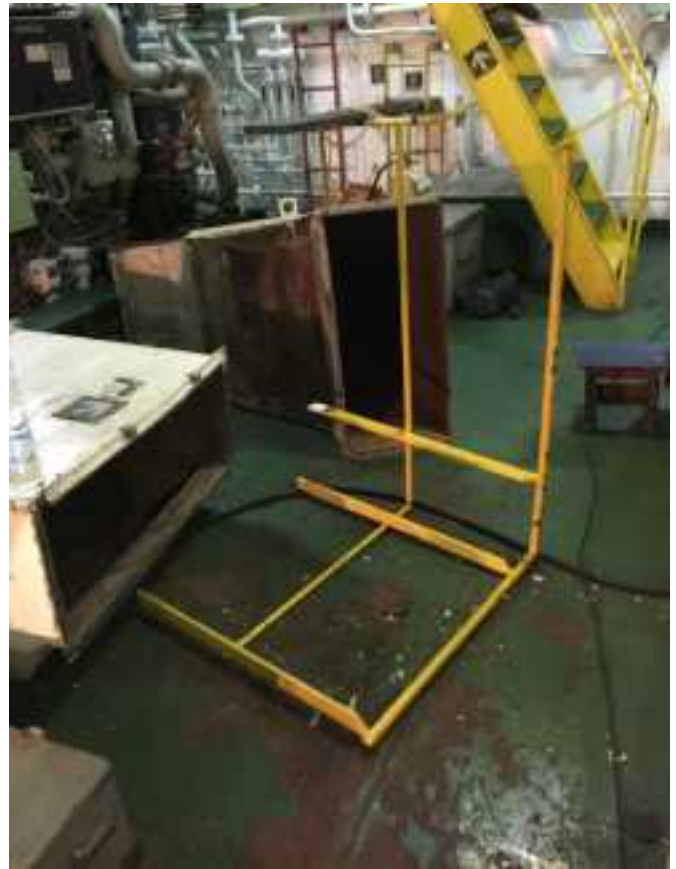
Removal of Railing in Engine room
