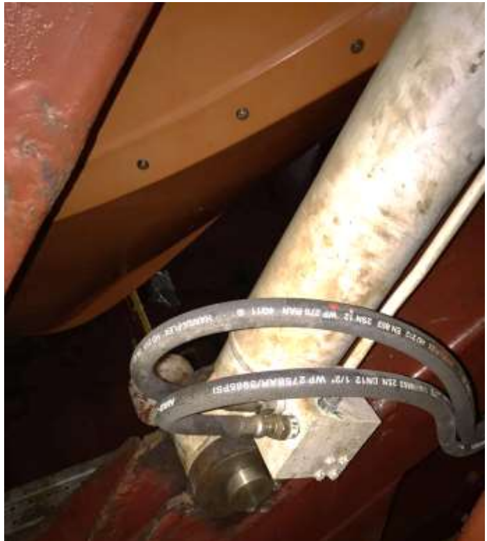
Bottom side of hydraulic cylinder after installation
