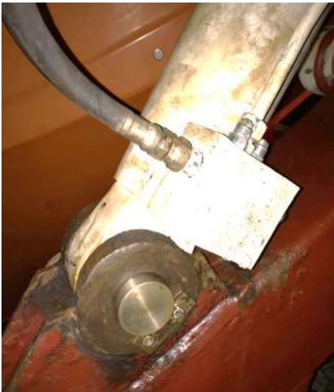
Bottom side of hydraulic cylinder after installation
