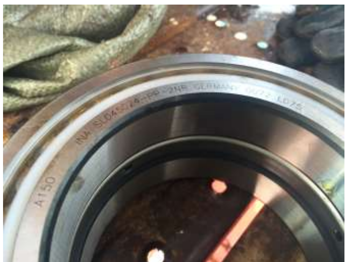
Existing collar plate found worn off
