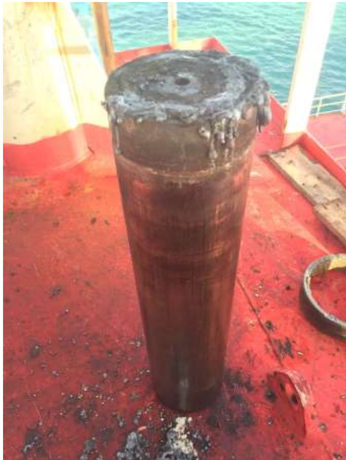
Extracted pin found in good condition
