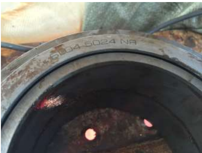
Existing collar plate found worn off
