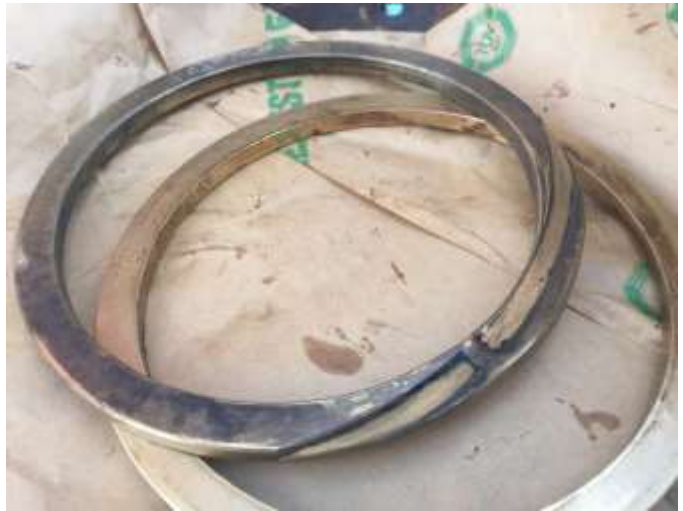
Existing collar plate found worn off
