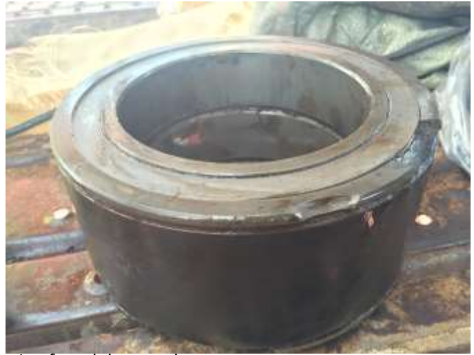
Existing extracted bearing found damaged
