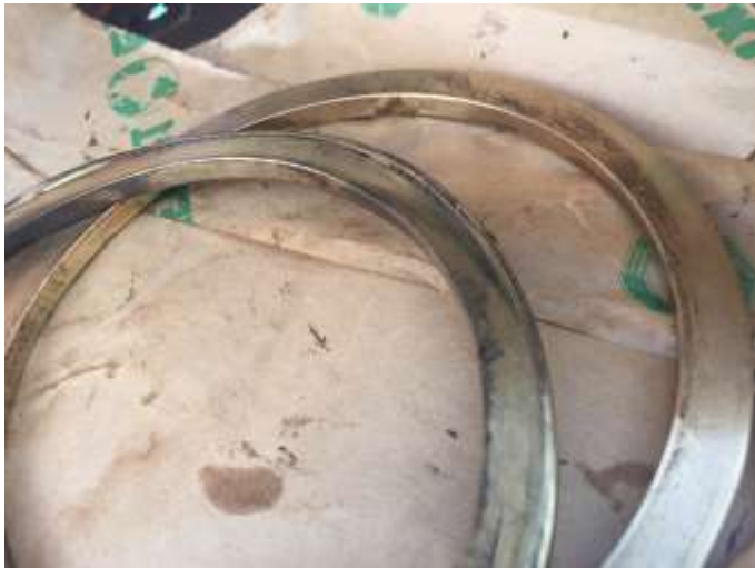
Existing collar plate found worn off
