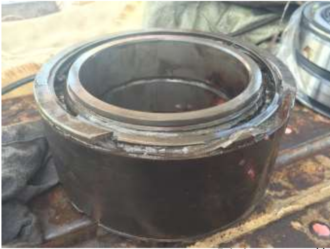
Existing extracted bearing found damaged
