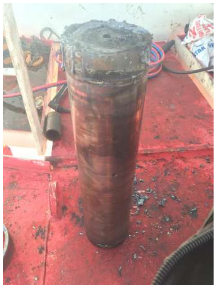
Extracted pin found in good condition
