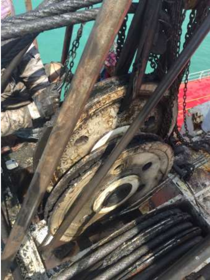
Re-assembled all roller sheaves back in position
