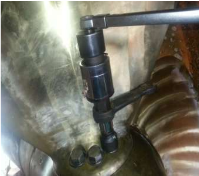
Torque tightening 600Nm on all the propeller blade bolts
