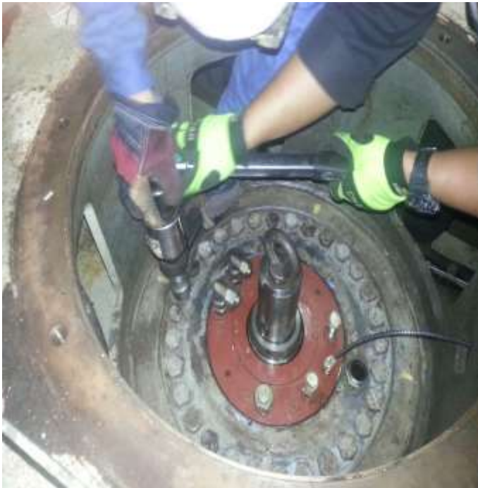
Torque tightening of 960Nm on all bolts
