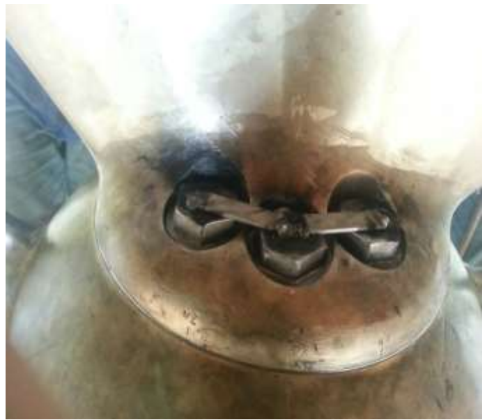
Spot welding on blade bolts locking plate
