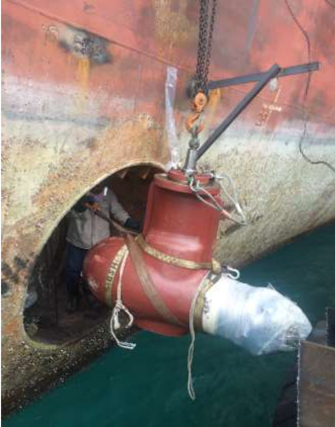
Transferred bow thruster unit from pontoon into thruster tunnel and positioned in place
