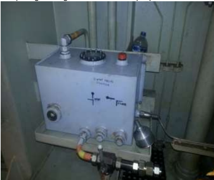
Filling up thruster oil and verified not leakage. And after carry out thruster pitch movement test.
