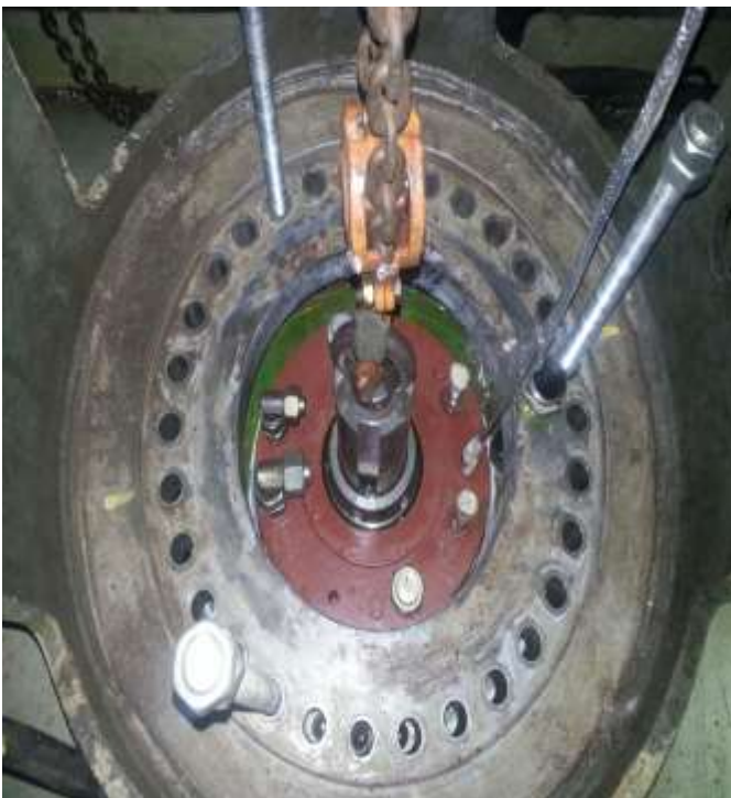
Transferred bow thruster unit from pontoon into thruster tunnel and positioned in place
