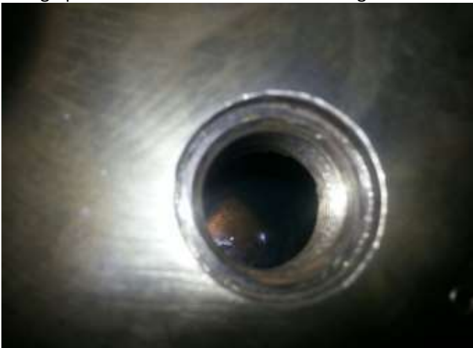
Filling up thruster oil and verified not leakage. And after carry out thruster pitch movement test.
