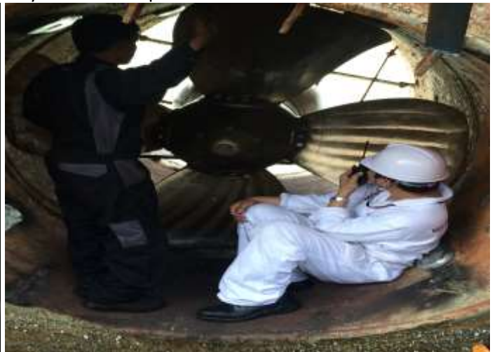
Filling up thruster oil and verified not leakage. And after carry out thruster pitch movement test.
