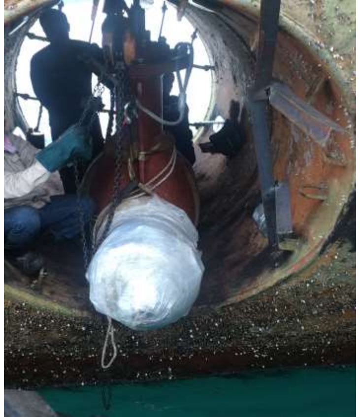
Transferred bow thruster unit from pontoon into thruster tunnel and positioned in place
