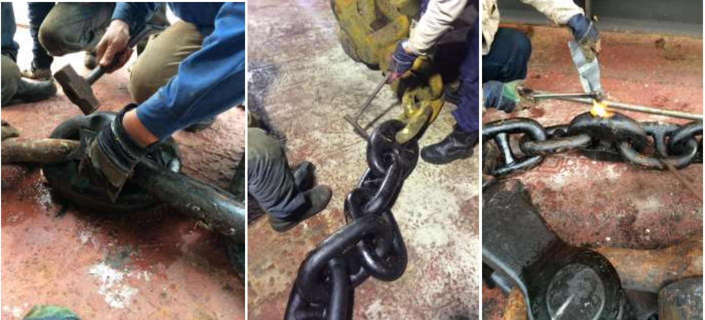
Fitting kenter shackle and apply lead to cover both pin hole.
