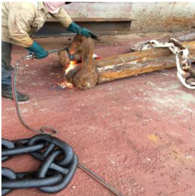
Cut off existing swivel piece connection
