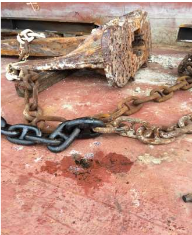
Anchor+ Anchor shackle+ Swivel+ End link+ Enlarged link+ common links
