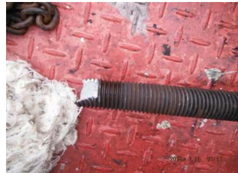
Continued extraction with hydraulic tools at 1000BAR pressure threaded stud broken and nut cracked fall off after Keep trying extraction the Sheave Pin were out.
