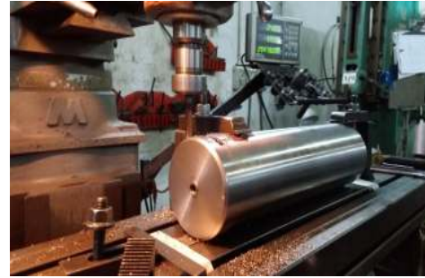
New pin were machined in work shop
