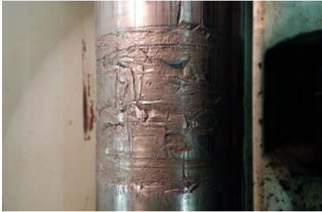
Pin were found with several damages and Chief Engineer advised bring to shore and machine a new pin.
