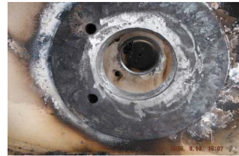
Carried out surface grinding of jib head sheave assembly.
