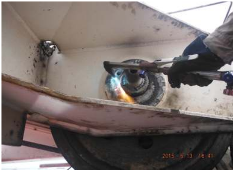
During the extraction nut were cracked and fall off
