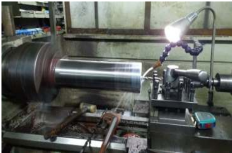
New pin were machined in work shop
