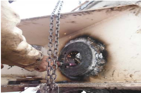
Carried out surface grinding of jib head sheave assembly.
