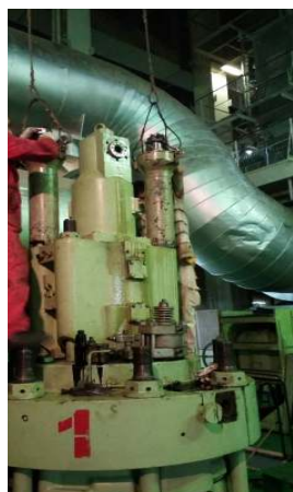
Hydraulic special tool were installed on exhaust valve and cylinder head to loosen the nut and dismount.
