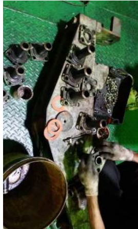
Lubricators were power brushed, cleaned, changed new 'O' rings/gasket and installed.
