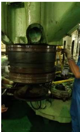
Existing exhaust valve were power brushed, cleaned, changed new 'O' rings applied Anti Seize Compound and installed.
