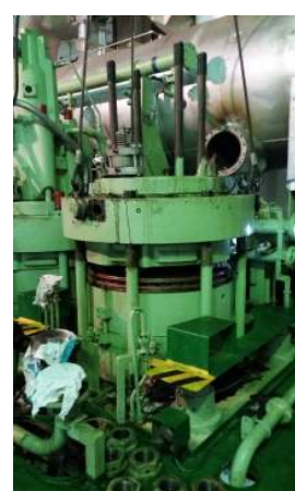
Hydraulic special tool were installed on exhaust valve and cylinder head to loosen the nut and dismount.
