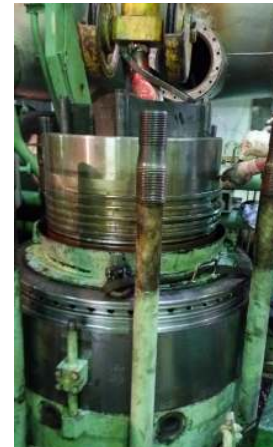
Ship's spare piston rod were installed in place and stuffing box 'O' rings were changed.
