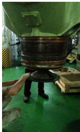
Existing exhaust valve were power brushed, cleaned, changed new 'O' rings applied Anti Seize Compound and installed.
