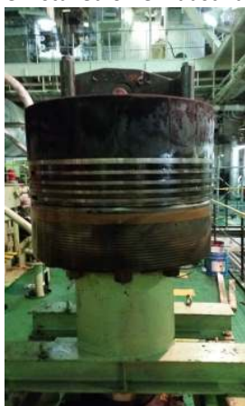
Decarbonized the thick carbon layer in the liner and extract the piston rod
