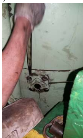
Removed all lubricators in order to extract the Cylinder liner
