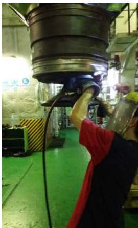
Existing exhaust valve were power brushed, cleaned, changed new 'O' rings applied Anti Seize Compound and installed.
