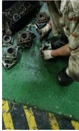
Lubricators were power brushed, cleaned, changed new 'O' rings/gasket and installed.
