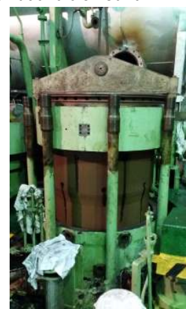
Removed all lubricators in order to extract the Cylinder liner
