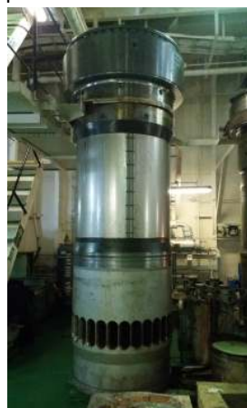
Decarbonized the liner casing, lubricator holes and ship's spare liner were installed with new 'O' rings and applied Anti Seize Compound.
