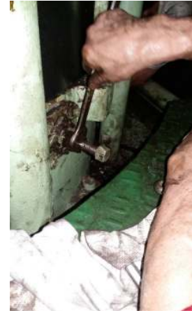
Lubricators were power brushed, cleaned, changed new 'O' rings/gasket and installed.
