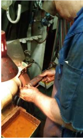
Lubricators were power brushed, cleaned, changed new 'O' rings/gasket and installed.
