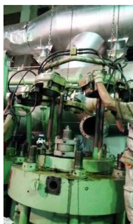
Hydraulic special tool were installed on exhaust valve and cylinder head to loosen the nut and dismount.
