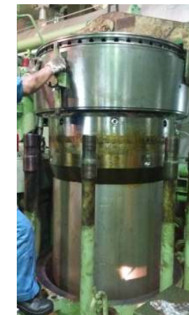
Decarbonized the liner casing, lubricator holes and ship's spare liner were installed with new 'O' rings and applied Anti Seize Compound.
