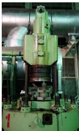
Hydraulic special tool were installed on exhaust valve and cylinder head to loosen the nut and dismount.
