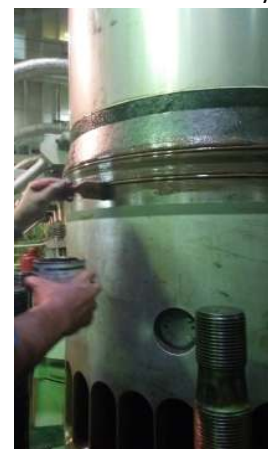
Decarbonized the liner casing, lubricator holes and ship's spare liner were installed with new 'O' rings and applied Anti Seize Compound.
