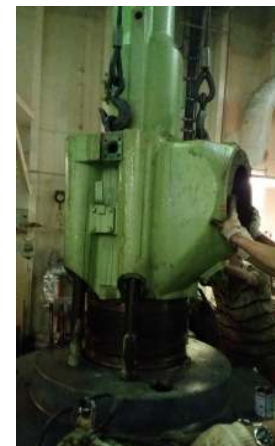
Existing exhaust valve were power brushed, cleaned, changed new 'O' rings applied Anti Seize Compound and installed.
