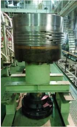
Ship's spare piston rod were installed in place and stuffing box 'O' rings were changed.
