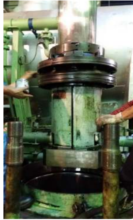
Ship's spare piston rod were installed in place and stuffing box 'O' rings were changed.
