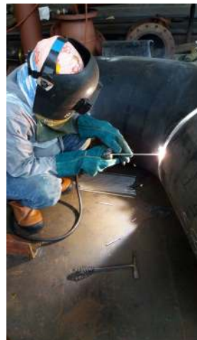
Carried out full welding on all the fittings, flanges and branches.
