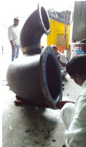
Upon completion carried out rubber coating in both pipes.
