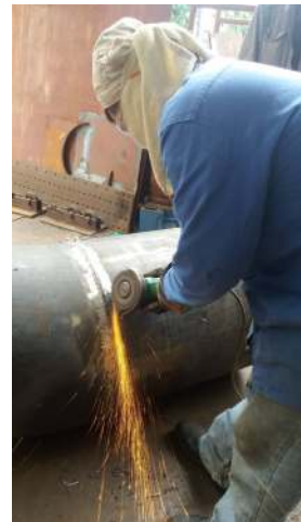
Well grinded on all the weldments and made smooth surface.
