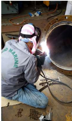
Carried out full welding on all the fittings, flanges and branches.
