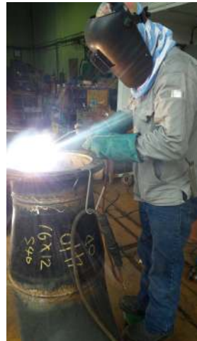
Carried out full welding on all the fittings, flanges and branches.
