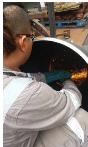
All pipes, fittings were cutted and grinded before fitting
