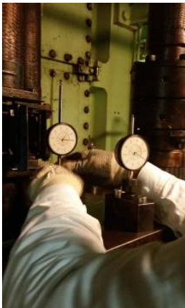
Upon Completion Fuel Injection Pump Timing Were Carried Out And Found Satisfactory. All Work Progress Was Inspected Witnessed Accepted By Chief Engineer With Satisfactorily.
