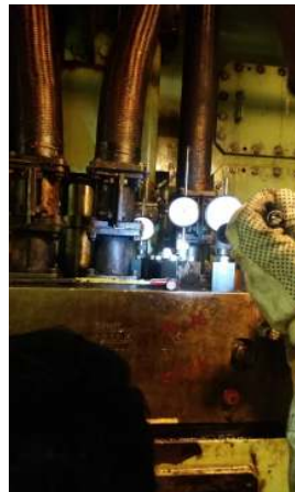
Upon Completion Fuel Injection Pump Timing Were Carried Out And Found Satisfactory. All Work Progress Was Inspected Witnessed Accepted By Chief Engineer With Satisfactorily.
