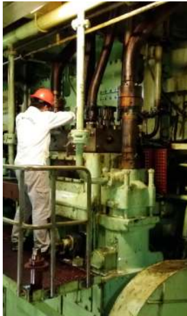
Cleaned the fuel oil pipes with diesel oil and installed and new gasket were changed
