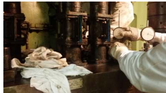
Upon Completion Fuel Injection Pump Timing Were Carried Out And Found Satisfactory. All Work Progress Was Inspected Witnessed Accepted By Chief Engineer With Satisfactorily.
