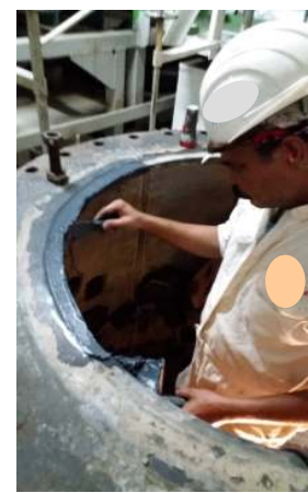
Applied New Rubber coating on all the spots
