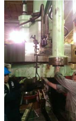
Liner was installed and new O rings were changed
