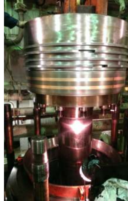
Liner was installed and new O rings were changed
