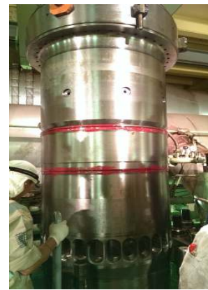
Reconditioned liner was installed with new O ring and calibrated
