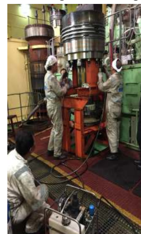
Piston crown mounted back and tighten
