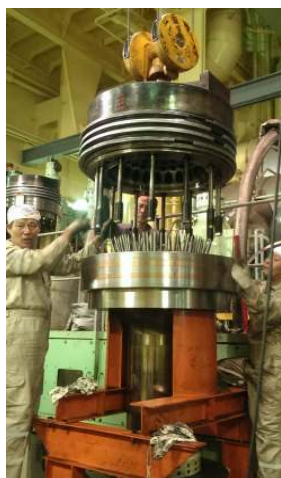
Piston crown mounted back and tighten
