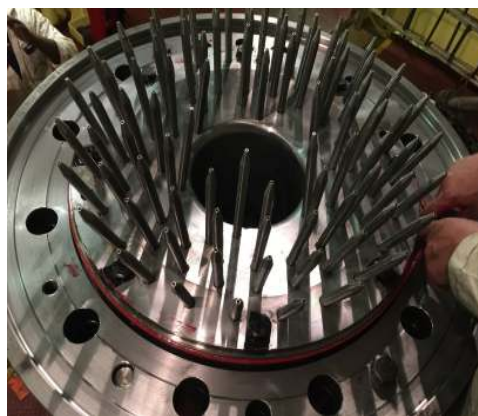
Nozzles cleaned and changed new O rings
