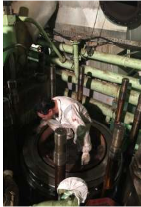
Piston was mounted back and changed new gasket
