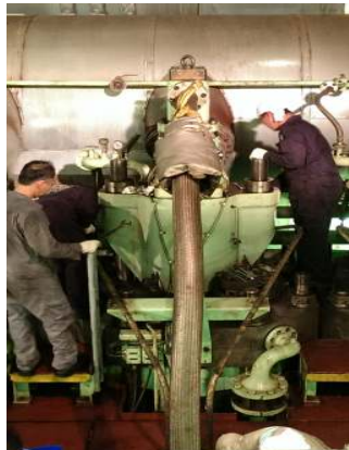
Removed all the connections. Hydraulic tool was installed and loosen the nut and cylinder head dismantled.
