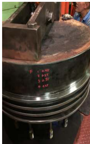
New piston rings were changed and calibrated
