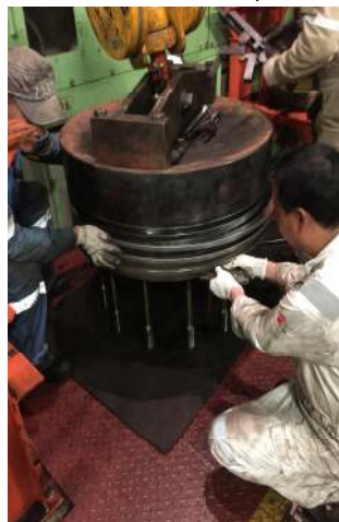
New piston rings were changed and calibrated
