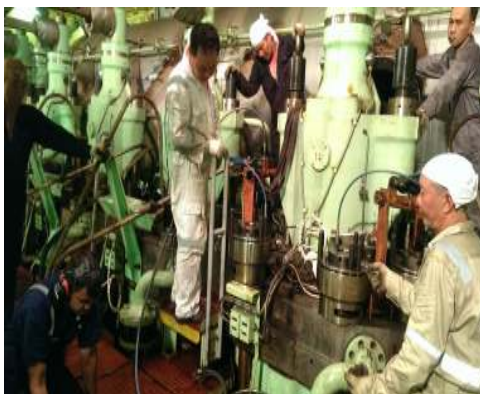
Removed all the connections. Hydraulic tool was installed and loosen the nut and cylinder head dismantled.
