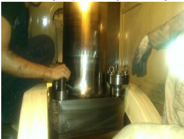
Remove piston nuts and withdraw the piston
