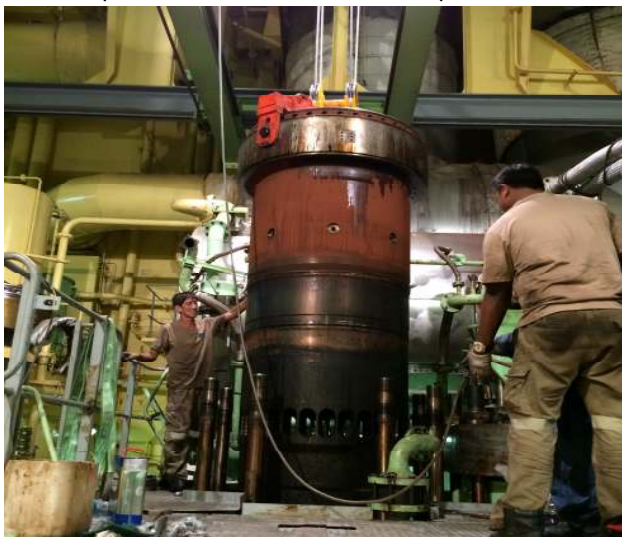
Extract liner and replace with spare unit.
