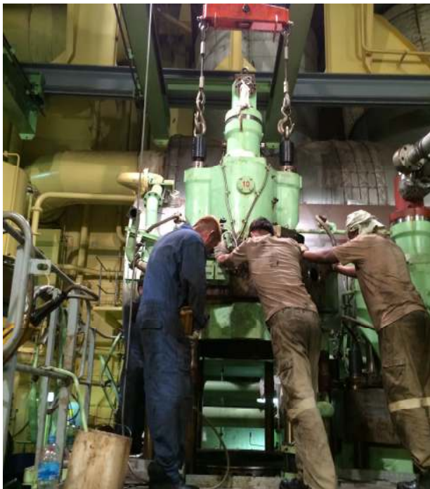
Reinstall cylinder cover and tighten nuts
