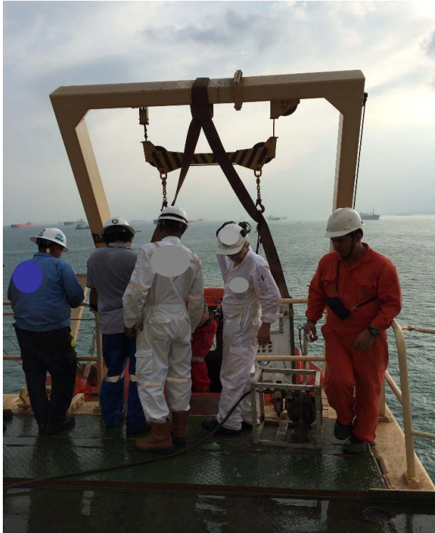
On load release test verified by class and ship rep
