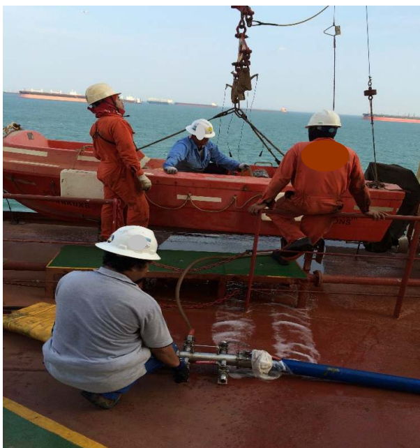
Filling water to water bags
